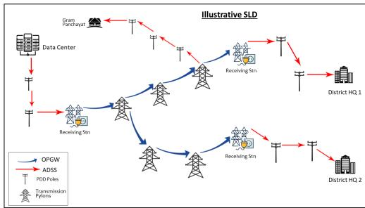
Figure 1: Indicative Diagram of the Network Design
